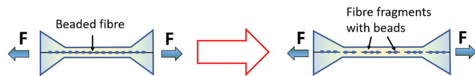
Figure 2. Schematic representation of a single fibre fragmentation test for a beaded fibre. Dog-bone shaped epoxy sample with embedded fibre is subjected to tension until fibre fragmentation occurs. Fibre fragments are hypothesised to have beads present on them.
