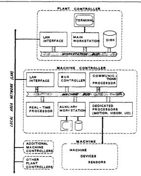
Figure 4. A Proposed Configuration for an Open-System Machine Controller
