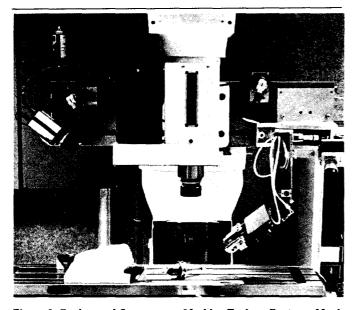
Figure 3. Devices and Sensors on a Machine Tool - a Dextrous Manipulator (DexMan), Cameras, and a Touch Probe (not shown) - the MOSAIC Project
